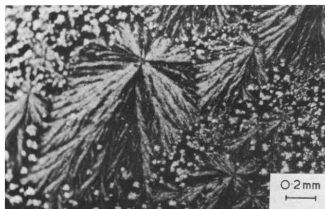
Figure 5 Micrograph as observed between crossed polarizers of spherulites with needle-like branches of silk fibroin crystallized by casting from aqueous solution at 20°C over a period of 7 days
